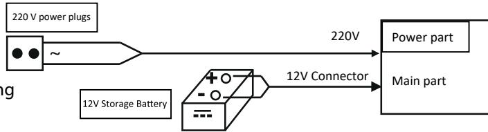
2. With "less voltage" protection, means, the 12v DC supply use after some time, the battery will decrease voltage, when the voltages decrease to 10.8v, TV will protect himself by not working automatically.
